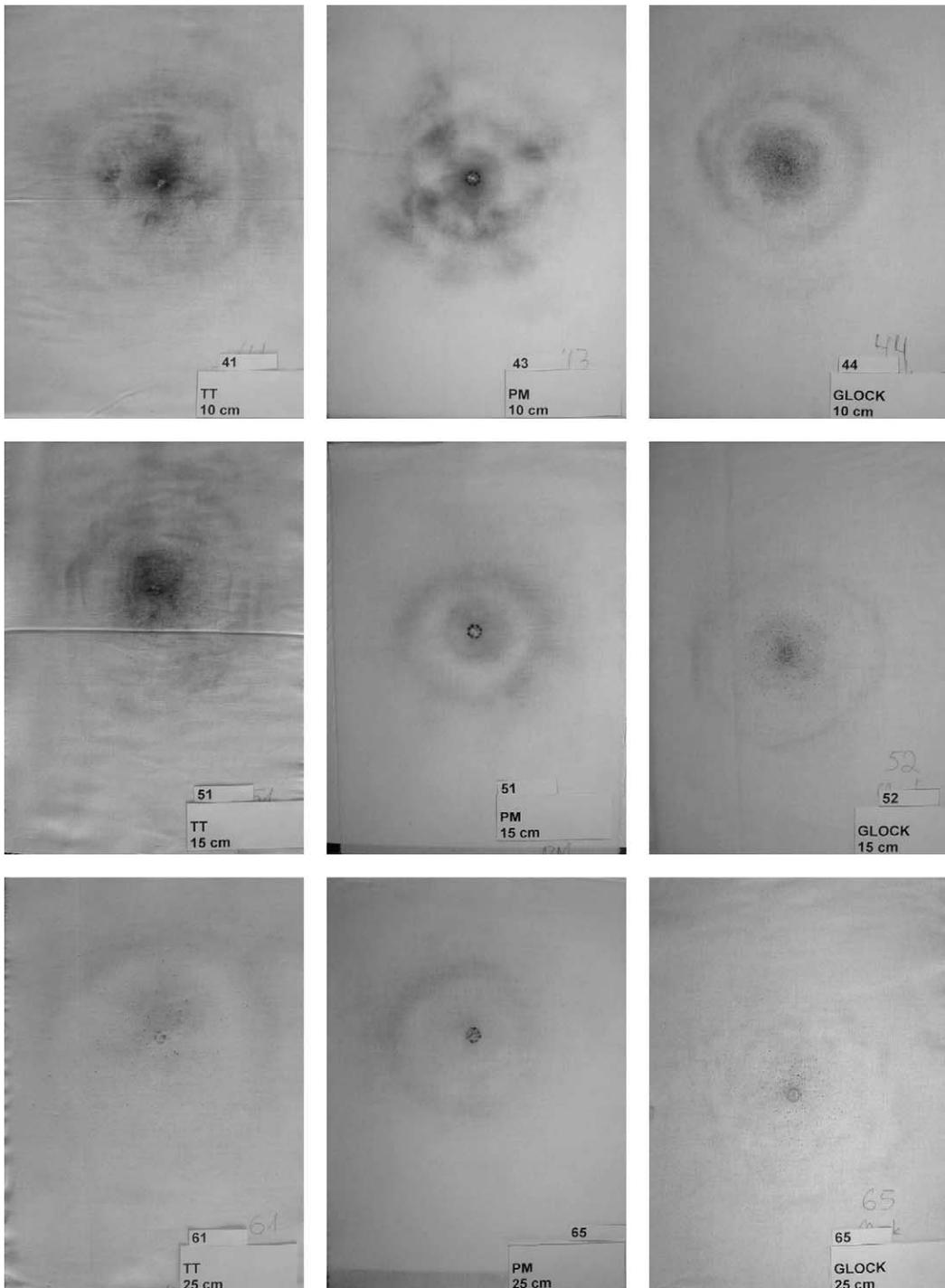
Fig. 1. Macroscopic pattern of soot and gunpowder residue particle distribution on cotton cloths.
